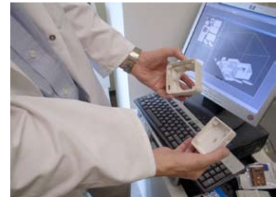
Fig. 5.15 Printed parts shown alongside CAD models
