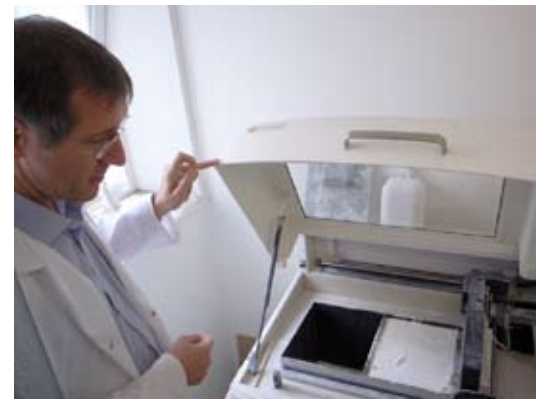
Fig. 5.14 Cases being printed using a rapid prototyping machine
