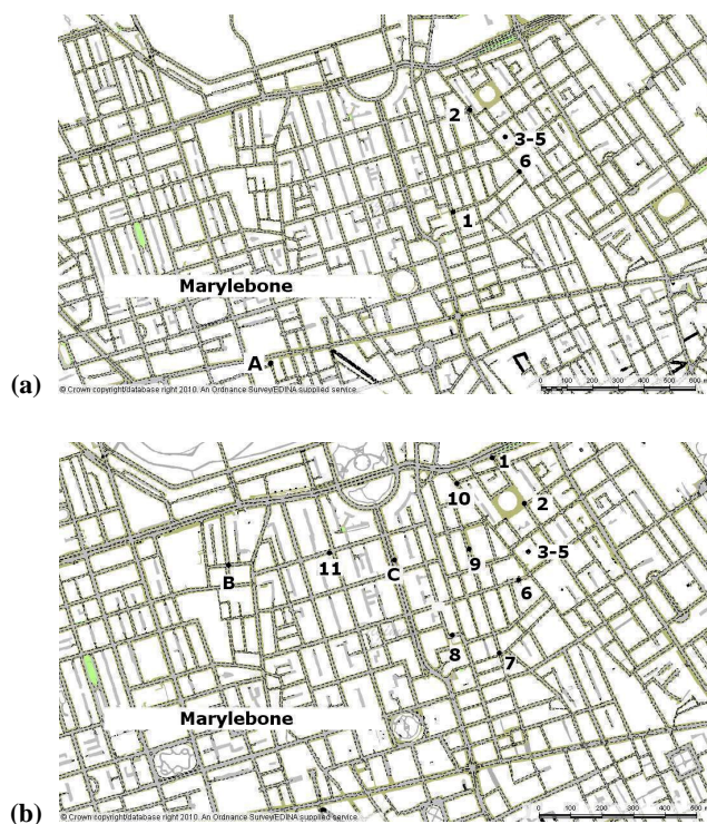
Fig. 1. (a) Experimental setup for the REPARTEE I. Source locations: A Receptor locations: 1 to 10. Note: receptors 3 to 5 located at heights 1.5 m, 160 and 190 m on BT Tower. (b) Experimental setup for the REPARTEE II. Source locations: B and C Receptor locations: 1 to 10. Note: receptors 3 to 5 located at heights 1.5 m, 160 and 190 m on BT Tower.
