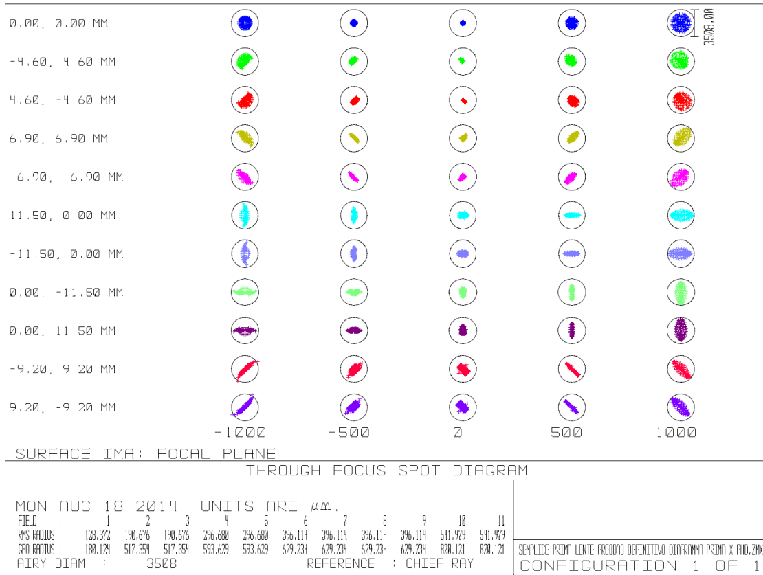
Figure 5.7: Through Focus Spot Diagram (TFSD) for all the eleven field shown in fig. 5.6(a)–5.6(b). The model shows the defocusing produced by a displacement of the focal plane. The model shows that the focus spot still falls within the Airy Disk (black circles in figure) for displacement between 1mm and -1mm , even for outer pixels.
