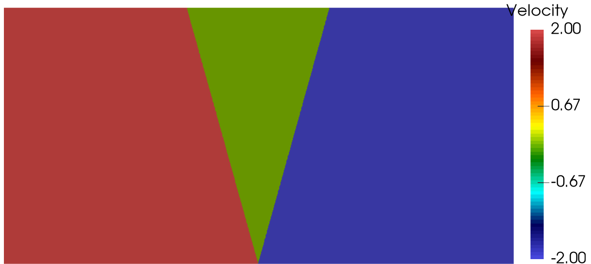
Figure 1.10 – Exact solution (1.26) of the dam-break problem (1.16) – (1.25). Representation of the velocity in two space dimensions, in the (x, t) -plane for t \in [0, 0.1] and x \in [-1, 1] .
