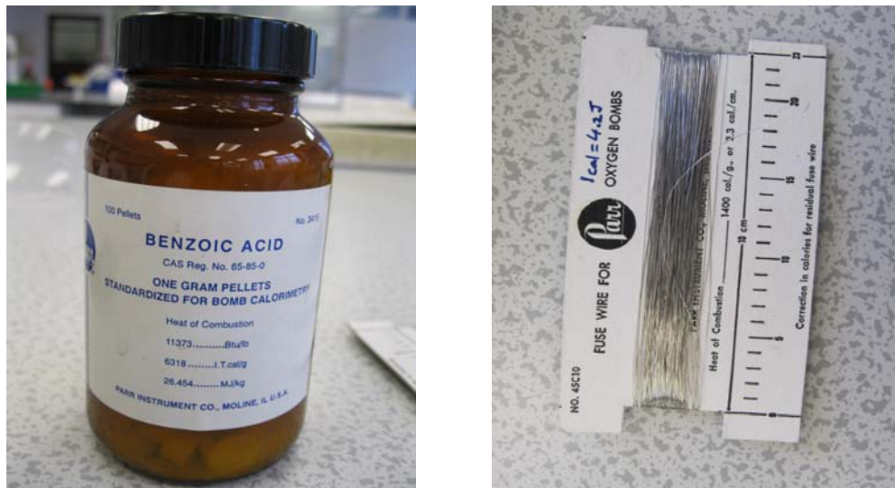
Figure 3.4: Benzoic acid and fuse wire for bomb calorimeter
