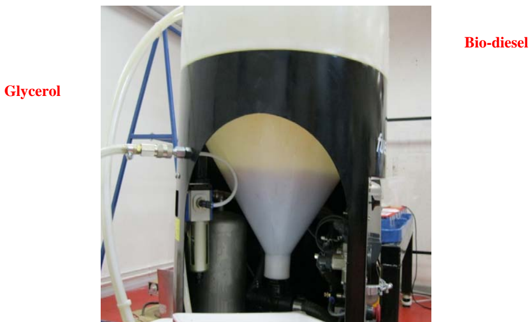
Figure 3.8: Separation of bio-diesel and glycerol
