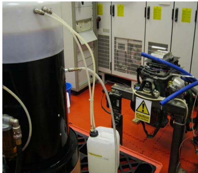
Figure A.6: Container holding mixture of methanol and sodium hydroxide connected with the system
