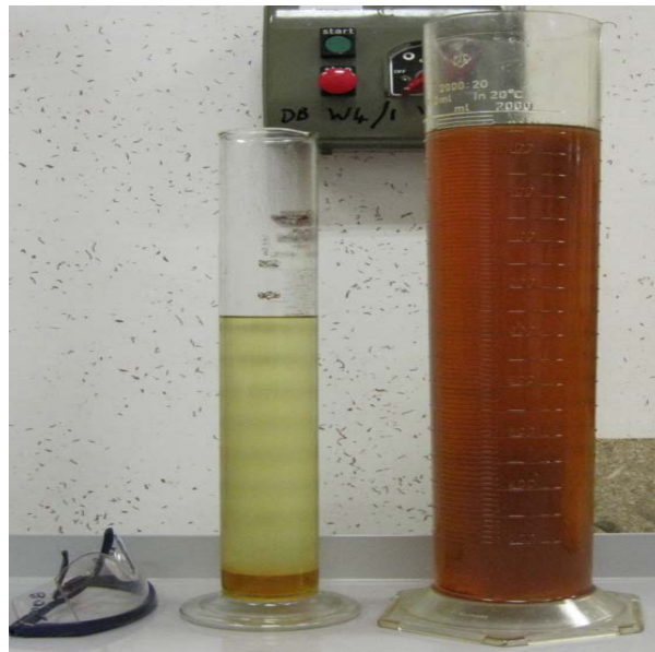
Figure 3.3: Bio-diesel and glycerol separation
