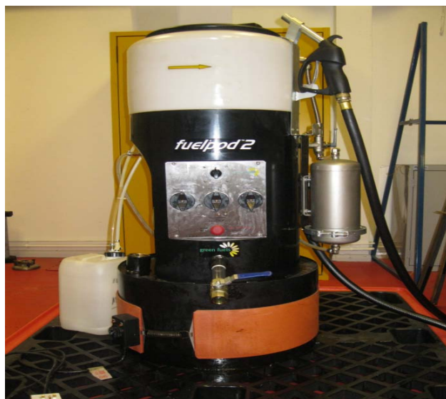
Figure 3.1: Fuelpod for transesterifying oils
