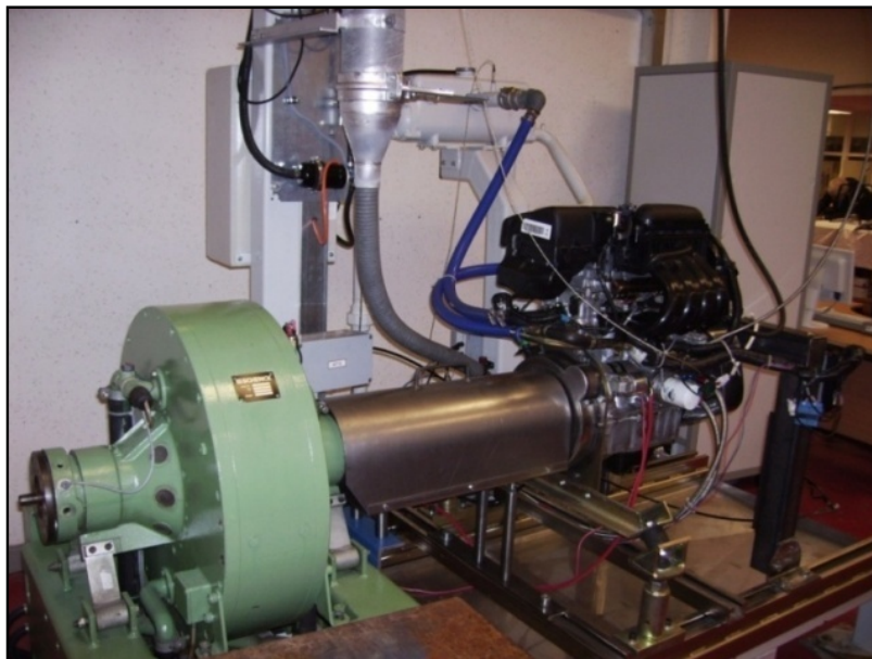
Figure B.1: Photo of test rig, Schenk dynamometer fitted with Ford Puma engine
