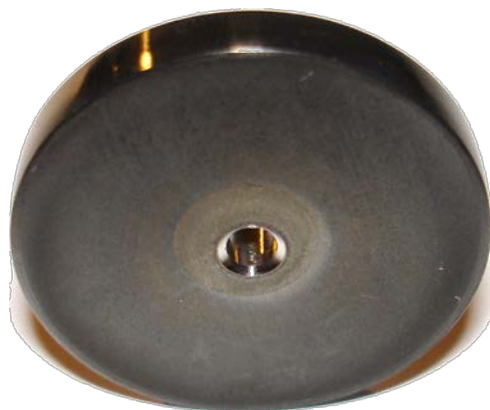
Figure 8.8 Sample Disc Manufactured from Forming Tool
