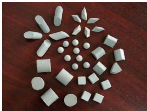
Figure 3.10 Various Abrasive Granule Shapes
