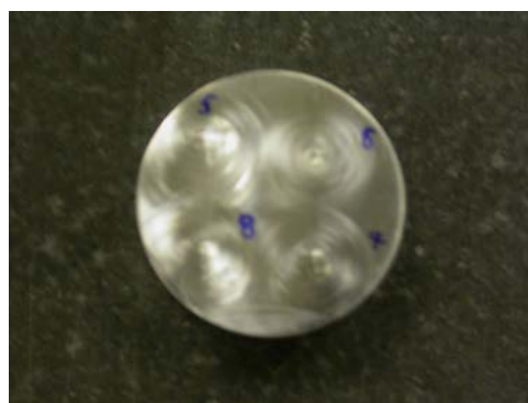
Figure 7.5 Influence Functions on 40mm Plano Cobalt Chrome Sample
