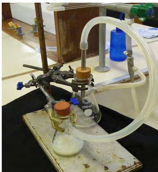
Figure 3-6. Equipment used to assess the effect of vacuum treatment upon AFEs. The size of air cells within the AFE was measured before and after treatment.
