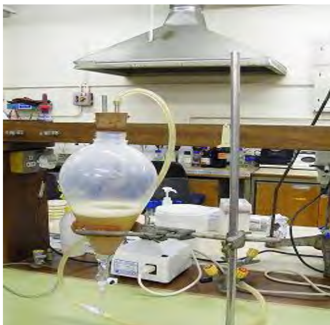
Figure 3-3. Separation of hydrophobin from the culture broth of Trichoderma reesei by foam fractionation
