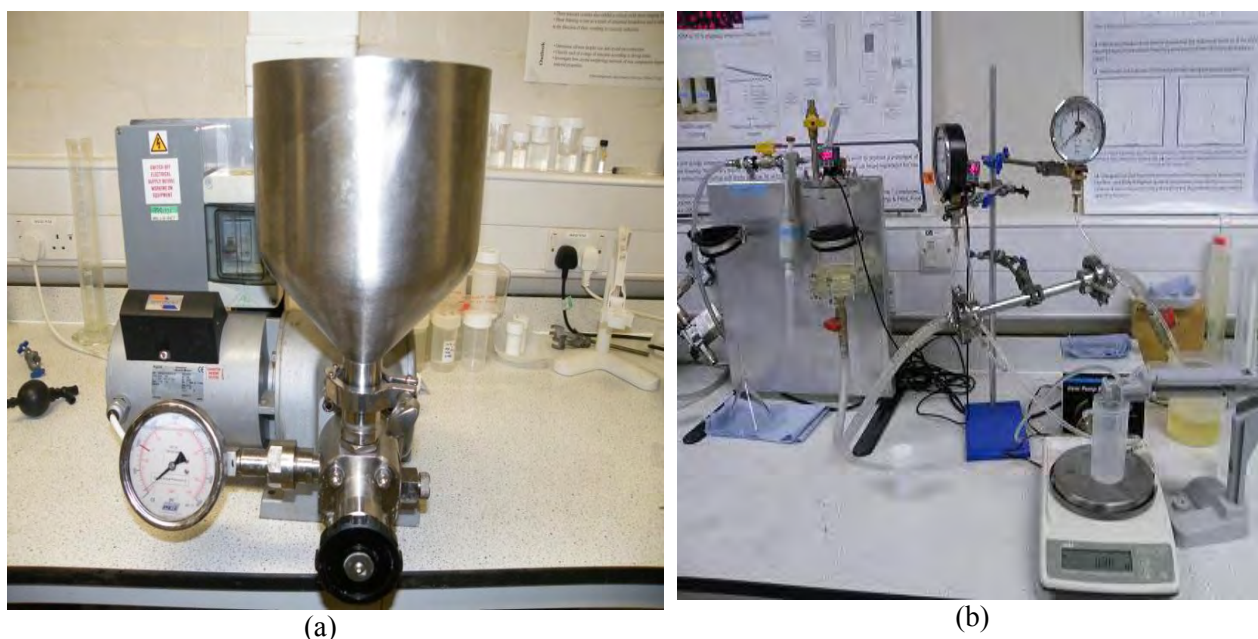
Figure 3-5. High pressure homogeniser (a) and cross-flow membrane emulsification set up (b).
