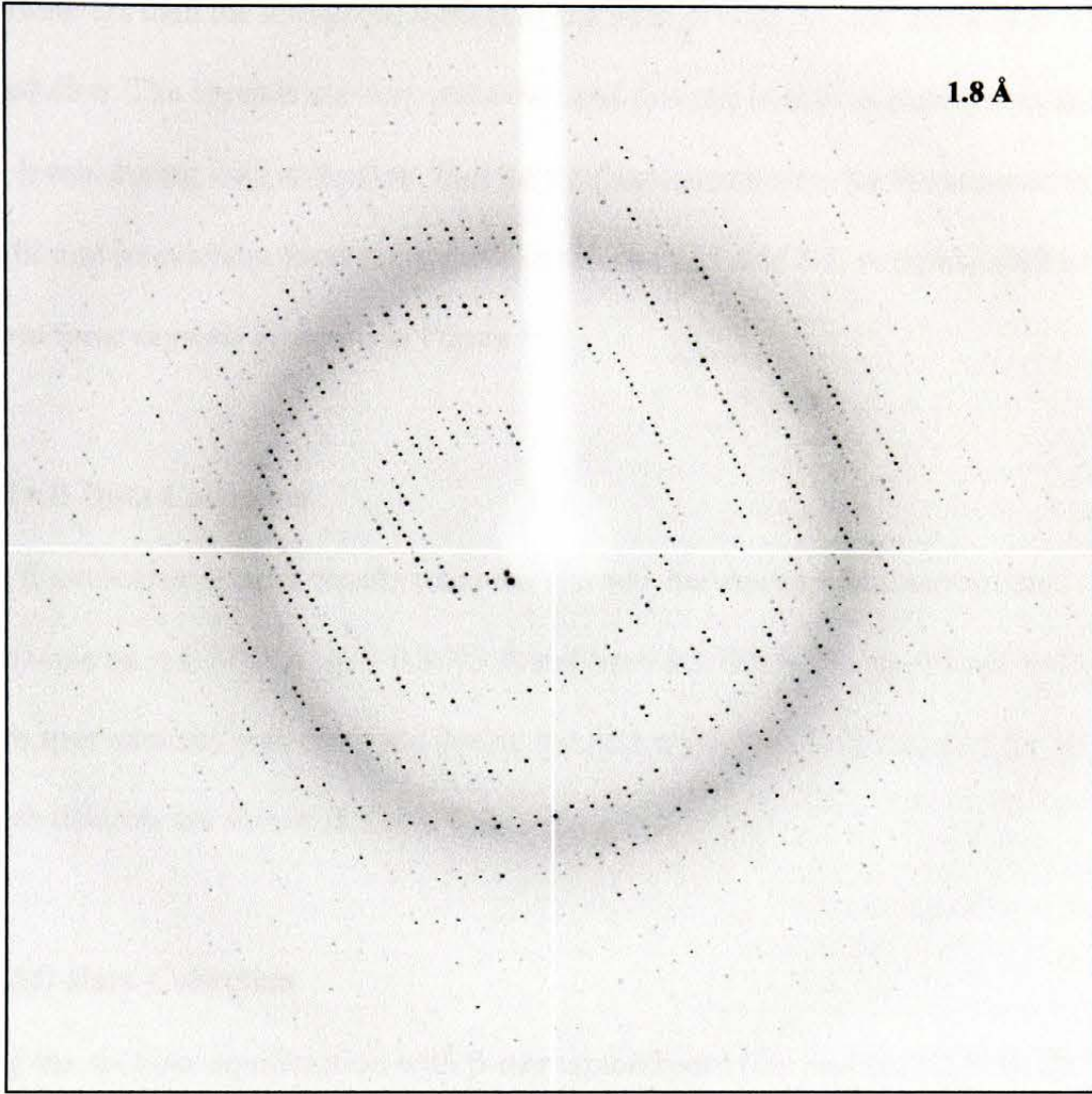
Figure 5.3. Example diffraction pattern from monoclinic crystal form, collected at beamline ID14-1, ESRF. Diffraction pattern from a 1^\circ oscillation. Resolution indicated in corner of image.
