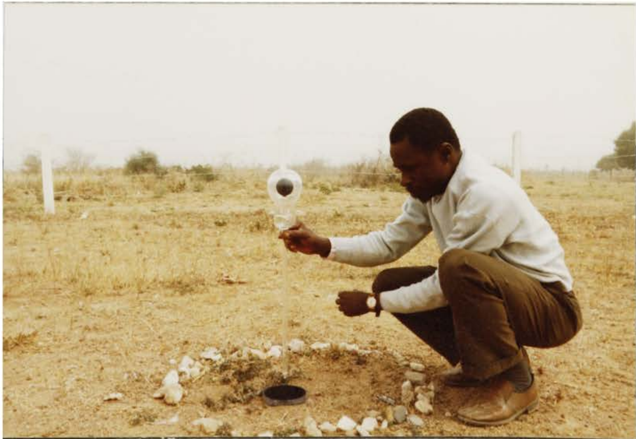
Plate 2.2 Gunn Bellani distillator - Bauchi. Note very dry ground surface in early February. Albedo = 0.35.
