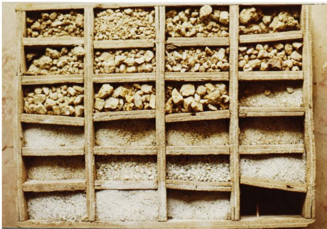
Plate 3.16. Drill cuttings from deep weathering area B. The hole has been drilled using a pneumatic down-hole-hammer rig, with the result that the more compact the rock, the finer ground is the sample. The rock dust in the final pocket represents fresh grade I material. The samples are arranged 'book fashion'. Note the absence of grade IV and V material, with a very thin grade VI.
