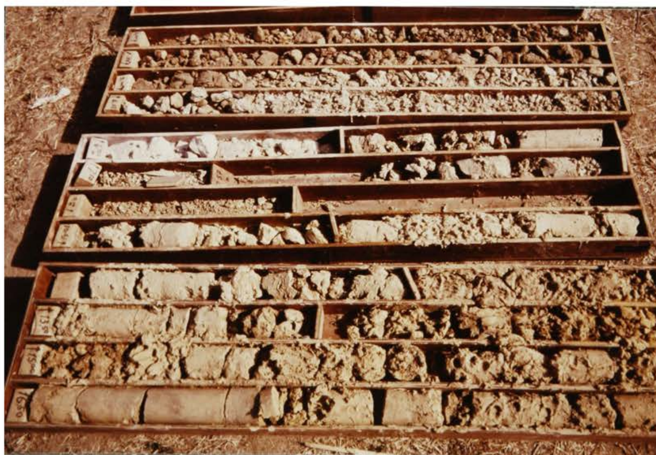
Plate 3.17. Extensive grade V and VI material from deep weathering area C. Cores have been obtained using dry drilling techniques. S.W.L. 15.5m.
