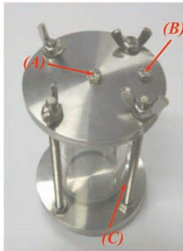
Figure 7.5: Vessel geometry. Points A , B and C , where tracer was located for the vessel motion measurement.
