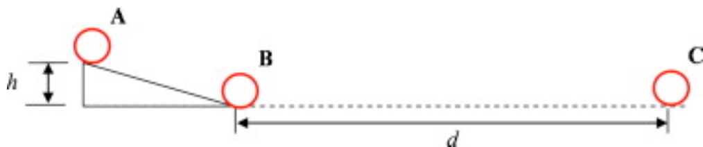
Figure 2.20: Setup for measuring coefficient of rolling friction for pharmaceutical tablets using a slope of height h and measuring the distance d travelled on a flat plane [98].
