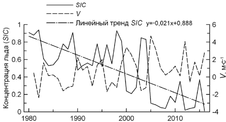
Fig. 3. Multi-year variation of the sea ice concentration and the wind speed meridional component averaged over the area 76 – 78° N and 42 – 62° E
