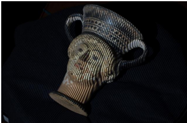
Figure 2. SmartScanHE C8 fringe projection scanner (above). Fringe projection scanning process on attic head vase (below, Antikensammlung Berlin).
