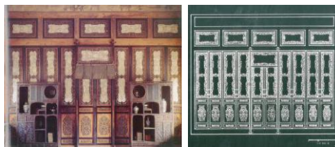
Figure 7. Photo and survey drawing of Taijidian
