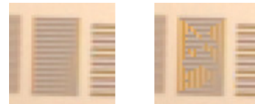
Figure 4. Artefact of the AHD algorithm. The maze-like structure on the right is an effect of the algorithm alternating between horizontal and vertical interpolation (Gózdź, 2009).
