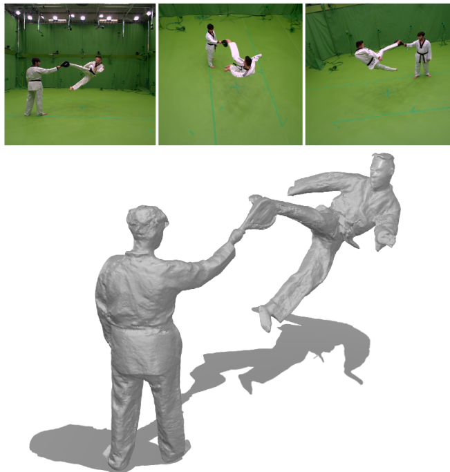
Figure 1. A challenging dynamic scene with fast motions and a mid-scale acquisition space, hence low image resolution on shapes in addition to motion blur. Temporal integration helps recovering highly detailed models.
