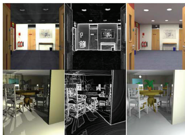
Fig. 9. The Corridor scene (top) and Tables scene (bottom). Left to right: the rapid image estimate, the saliency map and the selectively rendered final image. See Color palte 4
