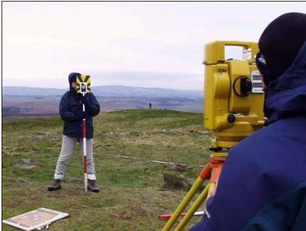
Plate 3.4. A Total Station survey (author's own photograph)
