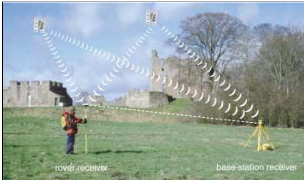
Plate 3.3. Illustration of the operation of a Digital Kinematic GPS System (after Ainsworth and Thomason 2003:9).
