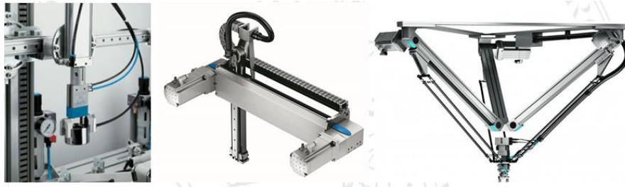
Fig. 2. Complex systems including significant pneumatic actuation.
