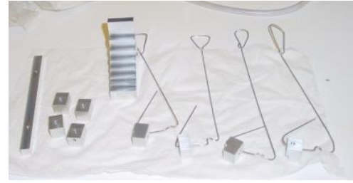
Figure 9. Artefact lined up for etching. After the etching process the single element were mounted into a fixed position (see Figure 6).
