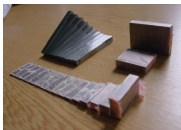
Figure 1. Mock-up of test object: set of Steel Slip Gauge Set M32, Calibration Grade 1 and Angle Block Set, length gauges to test step height and as length bar ( www.msclindustrial.co.uk ).
