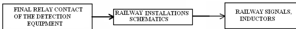
Fig. 5. The information from the execution relay is used in the already existing interlocking installations.
