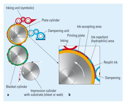
Fig. 1. Components of a printing unit.
