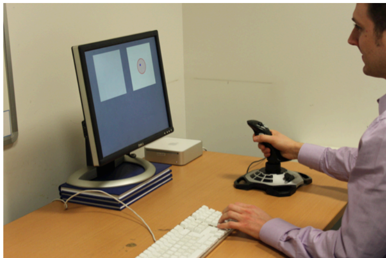
Figure 4.2: Physical set-up of the experiment. The tracking task is controlled with a joystick, and the typing task with the numeric keyboard.
