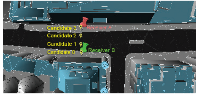
▲ FIGURE 8 Candidate user positions (in yellow) and true receiver positions (in red and green) in the shadow matching experimental verification
