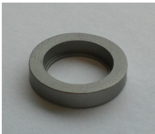
Figure 5.2 14mm diameter and 2mm length TiAl6V4 ring used in the gap model
