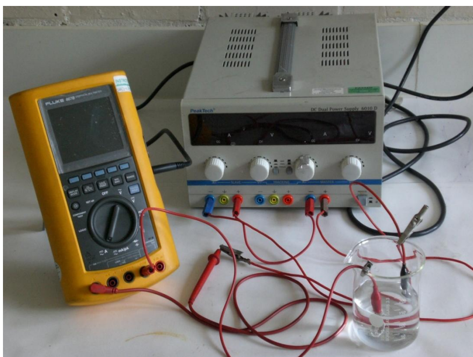
Figure 2.2 Equipment and setting for the electrochemical depositions of a CaP layer on the surface of titanium or tantalum discs.
