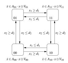
Figure 7: Hybridization: a nonlinear system is over-approximated by a hybrid automaton with an affine dynamics in each state. The transition guards indicate the conditions for switching between neighboring linearizations.
