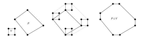
Figure 4: Adding a disturbance polytope V to a polytope P leads to a polytope  $P \oplus V$  with more vertices. The phenomenon is more severe in higher dimensions.
