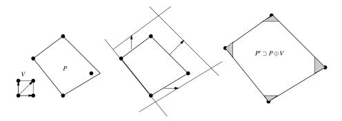
Figure 5: Pushing each face of P by the element of V which pushes it to the maximum. The result will typically not have more facets or vertices but may be a proper superset of  $P \oplus V$  (shaded triangles represent the over-approximation error).
