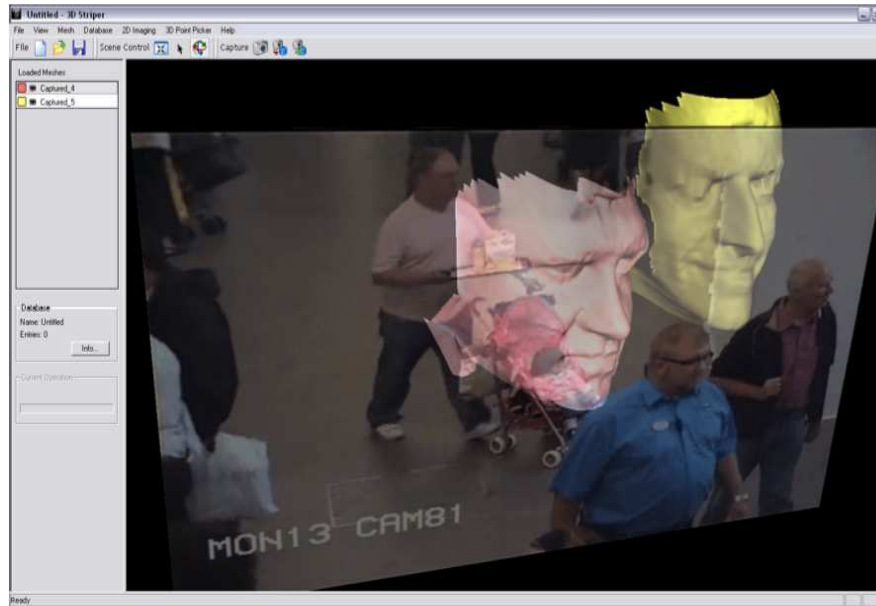
Fig. 9. Standard CCTV footage is projected on a 3D screen allowing the comparison of profiles
