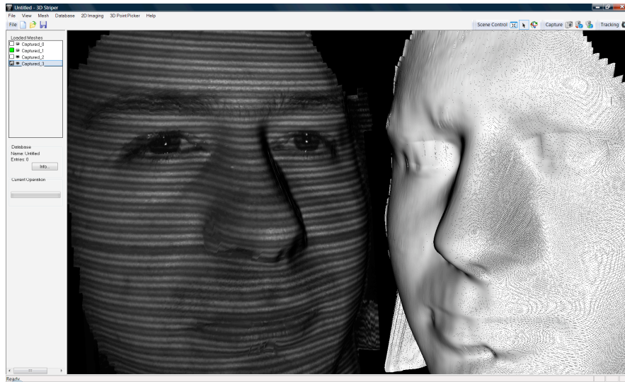
Fig. 1 Left, an example 3D model with NIR stripes on, right, wire mesh 3D model.
