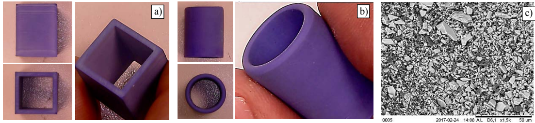
Fig. 3. Green printed parts of the photosensitive slurry of LTCC. Front, top and tridimensional view of them; (a) cubic geometry; (b) cylindrical; (c) SEM magnified view at x1.5k of the cubic geometry.
