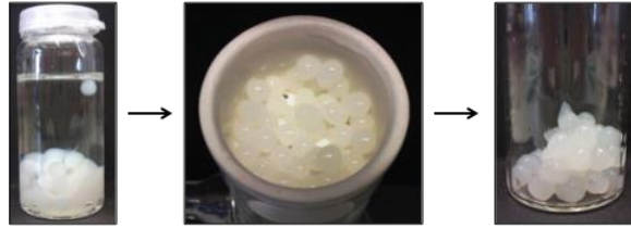
Figure 6. Na-Alg beads (4% w/v) obtained by dropwise addition in 0.5 M oxalic acid. Beads were washed with water several times (picture in the middle).
