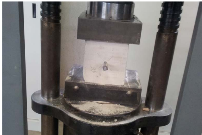
Figure 8 - Mortar sample with the inserted toothed nail ready for the torque test
