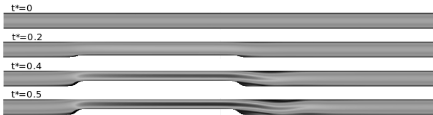
Figure 2.10: Velocity contour maps for different indentation values (extracted from [26]).
