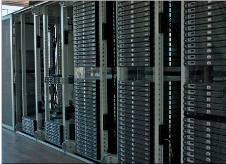
Figure 2.1: UPC's JFF supercomputer consists of 168 computer nodes with 2024 cores and 4.6 TB of RAM in total.
