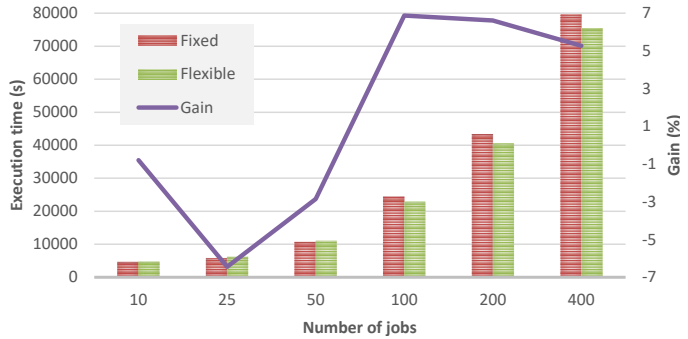
Fig. 7. Comparison between fixed and flexible workloads using asynchronous selection of action.
