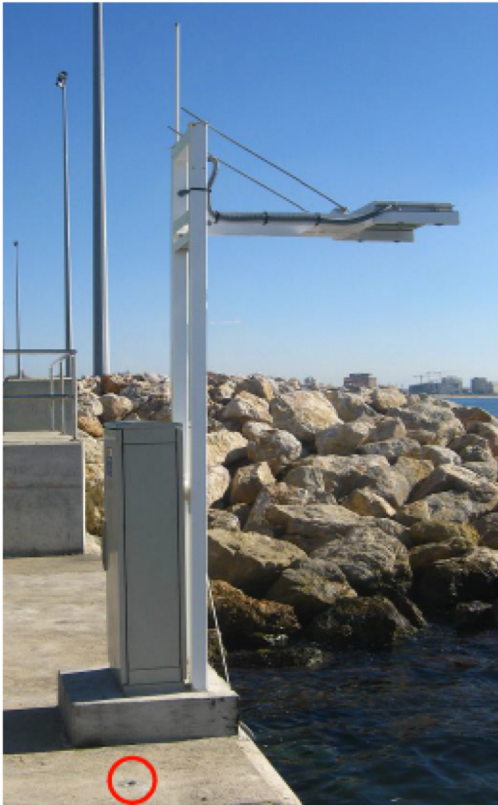
Figure 3.2: Photo of the GNSS Receiver and the geodetic reference level.
