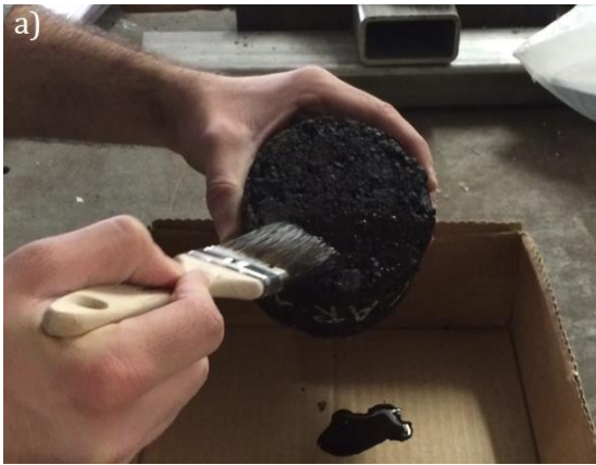
Figure 4. Application of bitumen emulsion (a). Preparing the molds for the SCHPC overlay (b).
