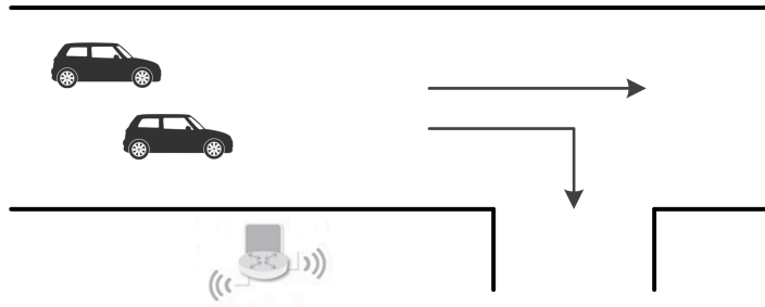
Fig. 5 Scenario to evaluate the exiting maneuver. It consists of a highway with an exit. The autonomous vehicles can either exit or continue in the highway based on their final destination. The RSU deployed as a Fog node assists with the contextual information.
