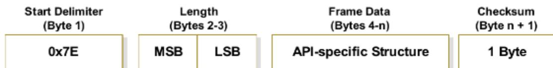
MSB = Most Significant Byte, LSB = Least Significant Byte
