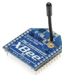
Figura 3.3 Xbee Series 1
