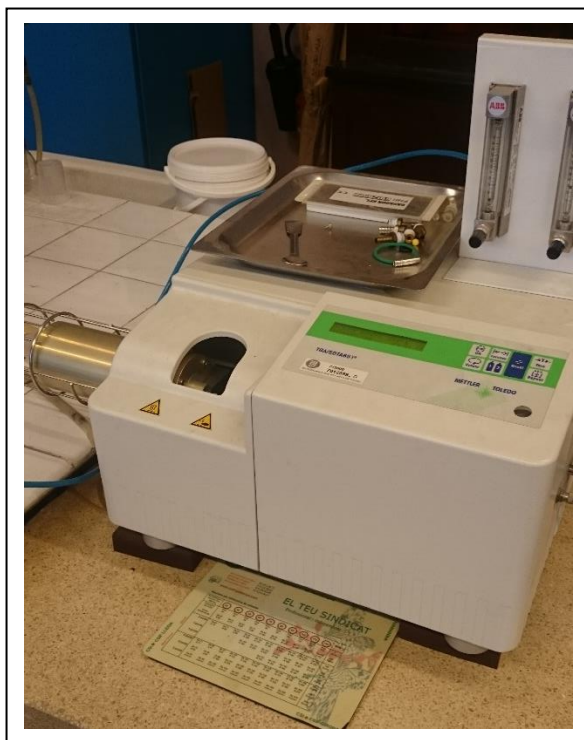
Figure 12. Thermogravimetric analysis machine.
