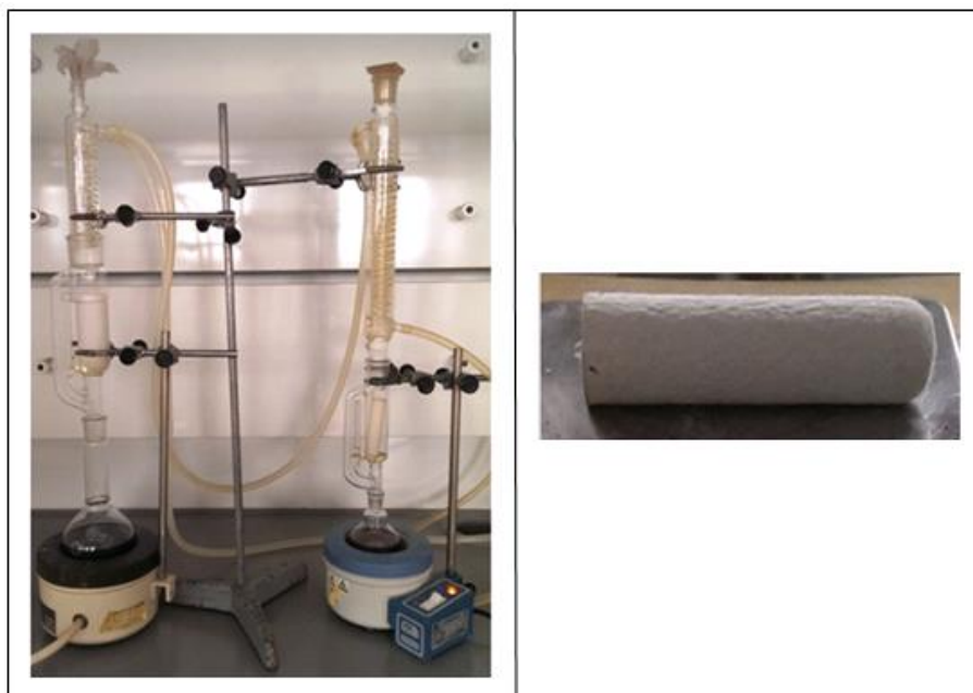
Figure 11: The Soxhlet extractor (left) and the filter paper thimble used (right).
