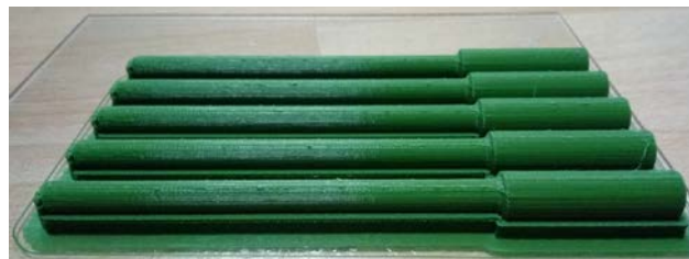
Figure 3. Printing tray with 5 test pieces printed with the same parameters
