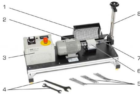
Figure 2. GUN WP 140 machine used to perform the different fatigue tests 1: Protective cover, 2: drive motor, 3: control center, 4: tools, 5: test pieces, 6: support, 7: test piece, 8: device to apply the load by rotating the black wheel on top.
