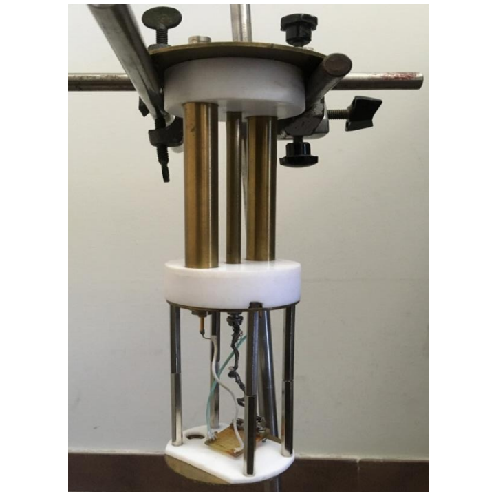
Figure(3.9): Sample holder for the chips carrying the interdigital electrode devices
