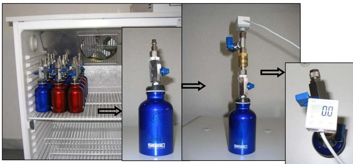
**Figure 3.4.** Incubation and biogas measurement during anaerobic batch tests (Ferrer *et al.*, 2004b)
