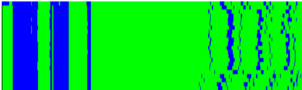
Figure 4.4.2: An example of a pre-processed image, where the blue color shows time spent in a parallel runtime and green color displays performing useful work.
