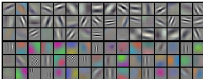
Figure 3.3.4: Illustration of the filters learned in AlexNet. Some are responsive of certain colors, others by certain structures. 12
