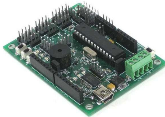
Figure 49. Picture of a BotArduino [62]
