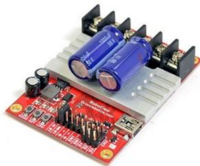
Figure 45. RoboClaw 2x15A motor controller [58]
