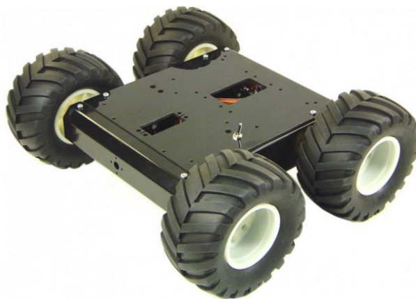
Figure 43. Lynxmotion A4WD1 chassis and wheels mounted kit [56]
