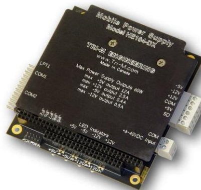
Figure 17. Picture of HE104+DX voltage regulator [46].
