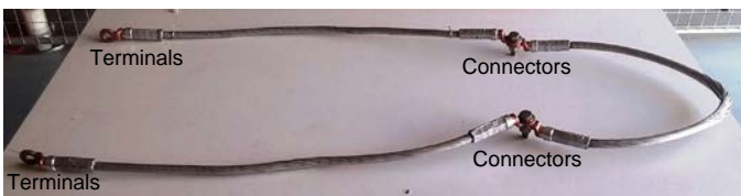
Fig. 5. AL-XZ1 1x120K conductor loop used during the short-circuit test.
