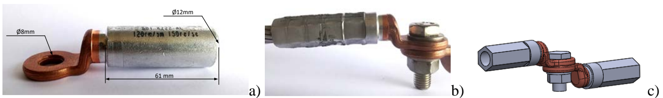
Fig. 1. YAT120AM130CP connectors. a) Before compression. b) After compression. c) CAD drawing including the bolting elements.
