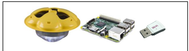
Fig 5. Smart Buoy case and electronics
