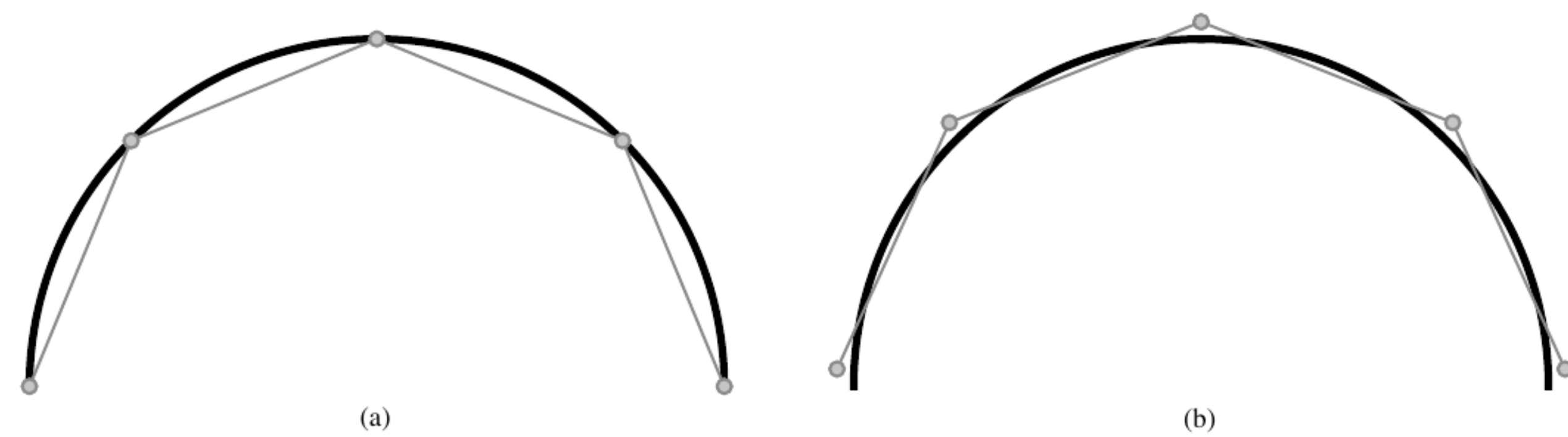
Linear meshes for a circular arc: (a) an interpolative mesh (nodes on top) and (b) a non-interpolative mesh (nodes floating around).
