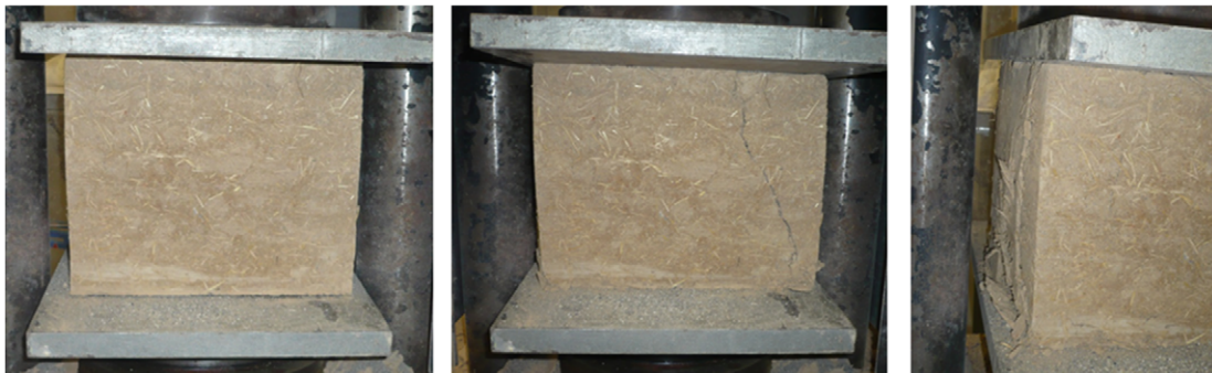
Figure 4. Rammed earth samples during compressive strength tests.
