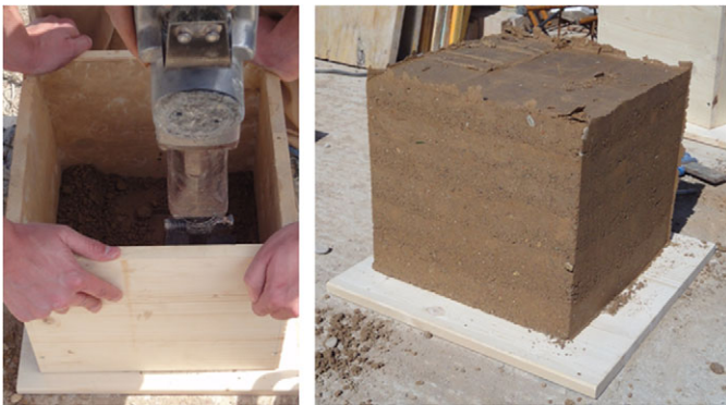
Figure 3. Rammed earth sample during manufacturing by layers (left) and finished (right).
