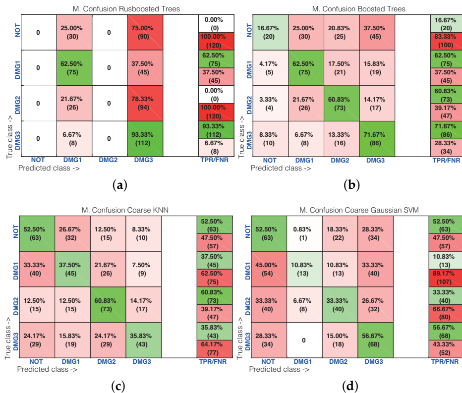
Figure 24. Confusion matrix machines with bad behavior. (a) Rusboosted trees; (b) boosted trees; (c) coarse k -NN; (d) coarse Gaussian SVM.
