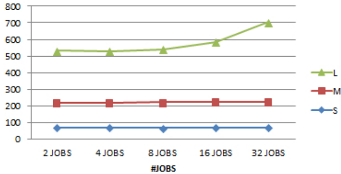
Figure 8. Response time (in seconds) for Small (S), Medium (M) and Large (L) size simulator instances for dynamic configuration of simulator
