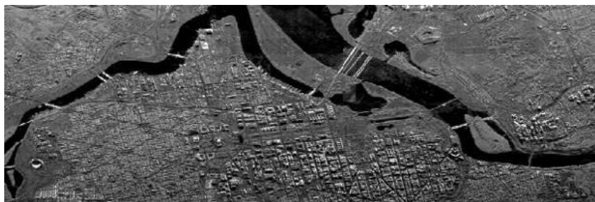
Figure 12: Strip map Synthetic Aperture Radar (SAR) of Washington DC.
