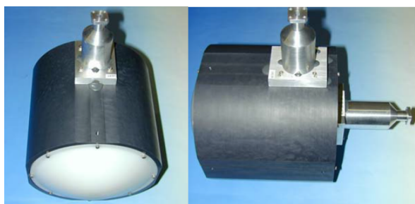
Figure 3. Corrugated horn with its Fresnel lens used in the Ka-band with the corresponding output waveguides for V and H polarizations.
