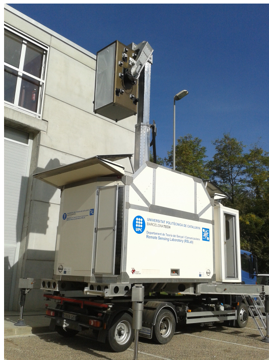
Figure 7. MERITXELL assembled to the telescopic robotic arm above the housing structure and the truck.
