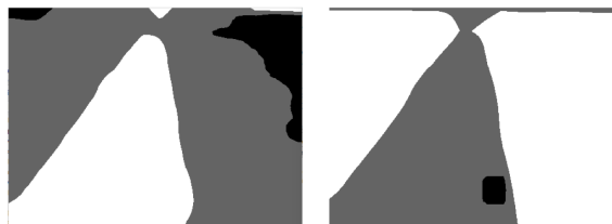
Figure 6: Resulting zones after converting the probabilities to markers and homogenizing the regions. For each class, road on the left and other on the right, there is a safe zone where the pixels sure belong to the corresponding class (white), a fuzzy zone where no markers will be defined (gray) and an unsafe zone that indicates the pixels that do not belong to the class (black).
