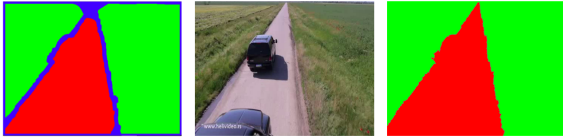
Figure 7: On the left, the resulting markers where red belongs to the class road , green belongs to the class other and blue determines the undefined regions. On the right, the segmented image after applying the watershed technique on the second frame (image on the center) using the markers obtained.
