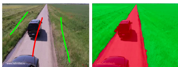
Figure 4: On the left, the first frame of a video sequence, where some seeds or markers have been defined for the road (red) and other (green) classes. On the right, the segmented image using the watershed technique with the defined markers.
