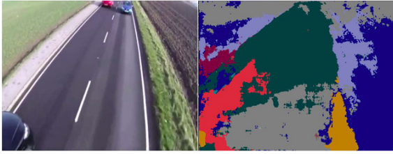
Figure 10: Image on the drones’ database, segmented with the original SegNet. Gray belongs to the sky, green to vehicles, yellow to pedestrians, dark blue to buildings, sky blue to trees, maroon to road and red to pavement.
